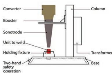
The process itself is very quick, a few seconds at most, it ends as soon as the ultrasounds stop, meaning the part can immediately be handled and continue to the next operation.
